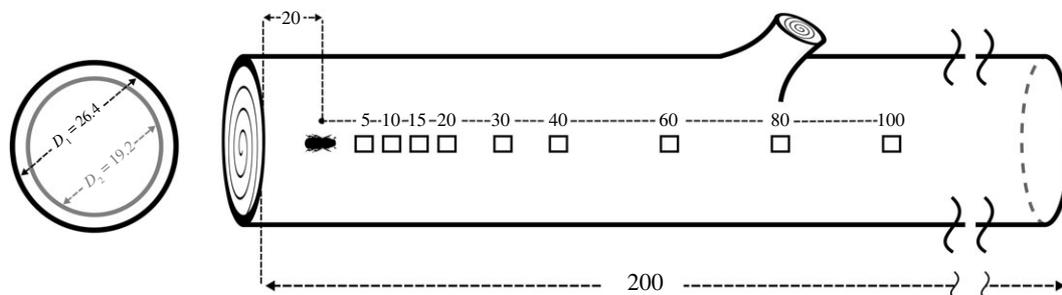
**Figure 2.** Experimental set-up for the analysis of sound propagation of two bark beetle species (*H. ligniperda* and *H. ater*) in wood.  $D_1$  and  $D_2$  are the average diameters of the *Pinus radiata* logs used for testing. A beetle was placed 20 cm from one end of the log. Stridulatory sounds produced by the individual were recorded at nonlinearly spaced distances from 5 to 100 cm. This procedure was repeated in the bark and phloem layer of each log. Dimensions in cm (not to scale).
