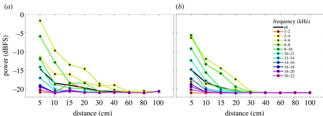
**Figure 5.** Average power decay with distance of the stridulations of (a) *H. ligniperda* and (b) *H. ater* estimated in frequency bands of 2 kHz for the entire dataset (phloem and bark). Most stridulations could be detected at their furthest reach using solely the 4–6 kHz frequency band, where spectral components were less attenuated. A version of these plots with error bars is shown in the electronic supplementary material, figure S3.
