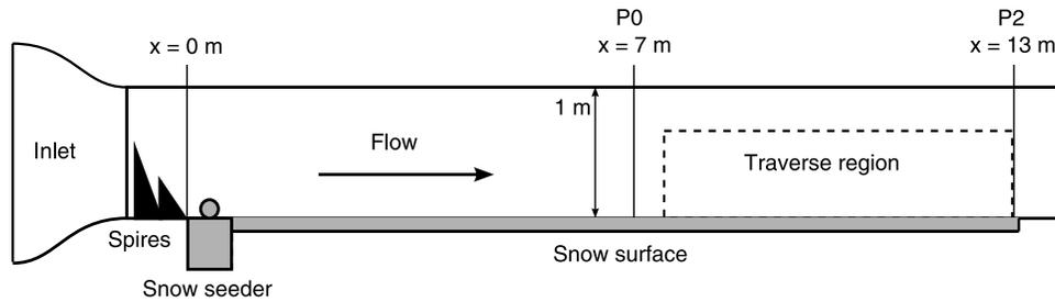
**Figure 2.** The working section of the Shinjo wind tunnel. Return section with fan and particle filters is not shown.
